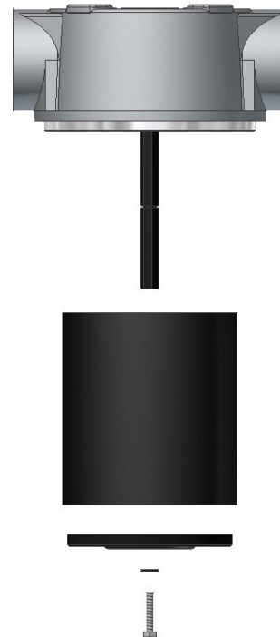
Figure C.3.2: Element and top plate removal.
